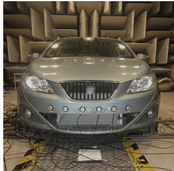
FIG. 8. (Color online) Six-actuator array attached to the front bumper of the vehicle.
